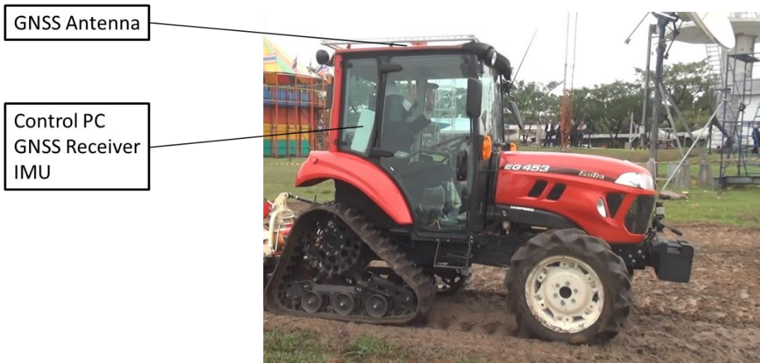
Robot Tractor under Demonstration Test (Yanmar EG453)
